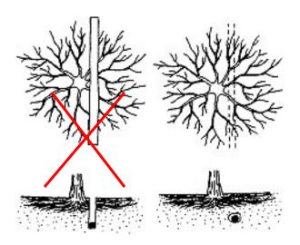
Tunneling below grade reduces root damage
